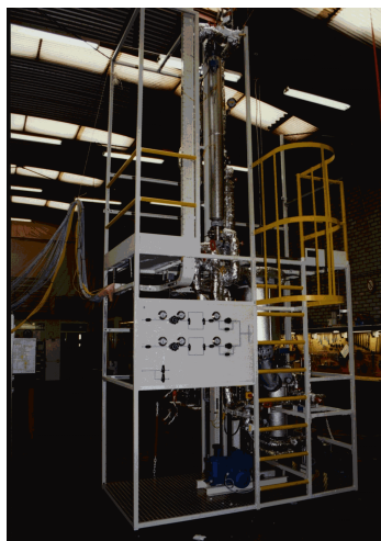
Pilot-scale reactor for testing monolithic catalysts
