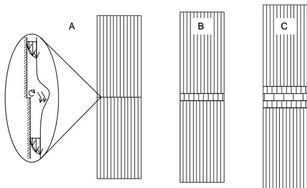
Better way of stacking monoliths might improve mixing and therefore increase G-L mass transfer without causing flooding
